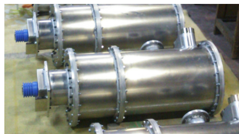
Figure 3: Picture of the storable inductance, which is installed below the kicker magnet.
