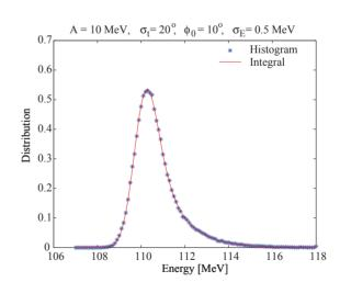
Figure 2: Energy distribution after the PETS for a beam with initial energy  $E_0 = 120 \,\text{MeV}$  and maximum loss of  $A = 10 \,\text{MeV}$ . Here the initial rms energy spread was taken to be 0.5 MeV. The blue dots are generated in a simulation the red line is the result of Eq. 11.
