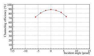
Figure 1: Single pass Channeling efficiency as function of protons incident angle. It is given by the fraction of deflected beam in a angular range of 2  $\mu$ rad centered on the red points. To be compared with Fig. 3 shown in [11].
