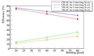
Figure 4: Single pass Channeling and Volume Reflection efficiency for 7 TeV impacting protons with  $\theta_{IN}$  < 1  $\mu$ rad, for different crystal lengths. Solid and dashed lines are obtained using the crystal routine implemented in SixTrack and the analytical code described in [1], respectively.
