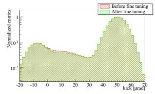
Figure 2: Distribution of kicks given by the interaction with a bent crystal, from where it is possible to calculate the Nuclear Dechanneling length through an exponential fit that ranges from  $\sim 10$  to  $\sim 30 \,\mu \text{rad}$ , as explained in [11]. What obtained before and after the fine tuning of the free parameters involed in the Nuclear Dechanneling model is shown in red and green, respectively.
