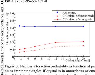
Figure 3: Nuclear interaction probability as function of particles impinging angle: if crystal is in amorphous orientation (blue), in channeling orientation before the routine upgrade (red dashed) and after (red solid). To be compared with Fig. 6 shown in [12].
