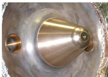
Figure 4: Cathode assembly after Ebeam welding.
