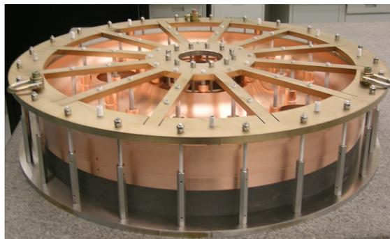
Figure 3: Cathode end cap in brazing fixture.
