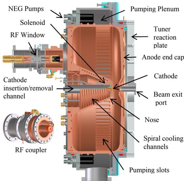
Figure 1: VHF Gun in cross section.
