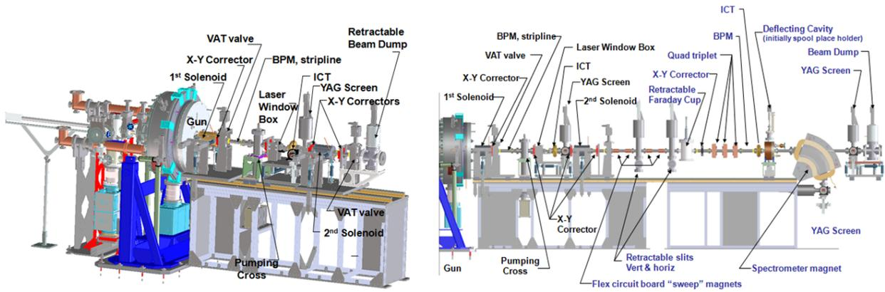
Figure 1: APEX layouts with main components in evidence. Left: Phase 0. Right: Phase I.
