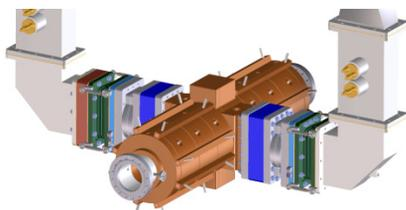
Figure 6: CAD view of the modified ANL-AWA 1.3 GHz accelerating section.
