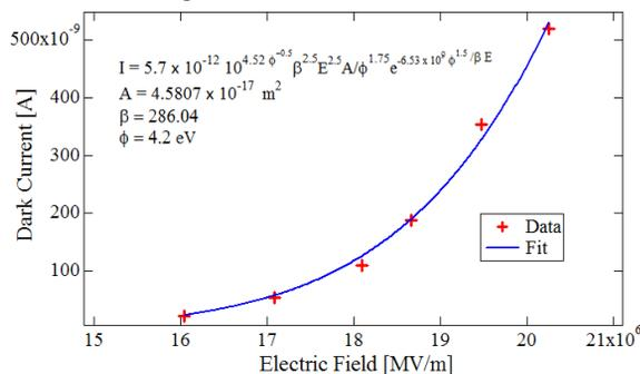
Figure 8: Example of dark measurement (DC) at APEX. At the nominal gradient of 19.5 MV/m the DC is ~ 350 nA satisfying the requirement of Table 1.
