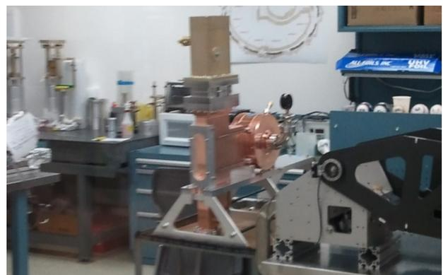
Figure 4: The transverse deflecting cavity ready for installation.
