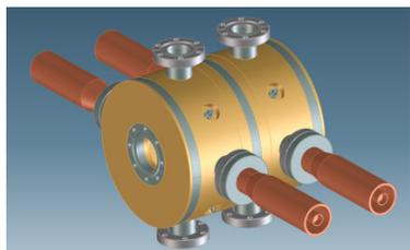
Figure 5: CAD view of the APEX 1.3 GHz buncher.
