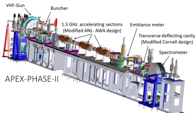
Figure 2: APEX Phase II layout.
