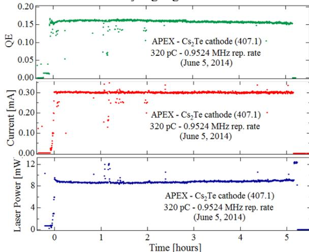
Figure 7: QE measurement for a Cs<sub>2</sub>Te cathode. The 1/e lifetime measured from 2 to 5 hours is ~ 2.94 days. More than 5.5 C were extracted. For comparison this is the charge extracted in ~ 13 days at FLASH.
