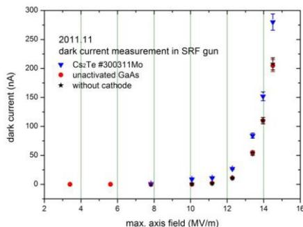
Figure 5: Dark current from SRF gun with Cs<sub>2</sub>Te, GaAs, respectively.
