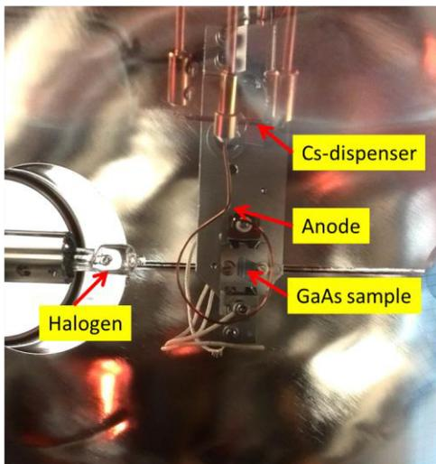
Figure 4: Insight view of the GaAs preparation chamber.
