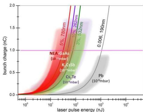
Figure 1: The compare of different photocathodes for superconducting rf gun.
