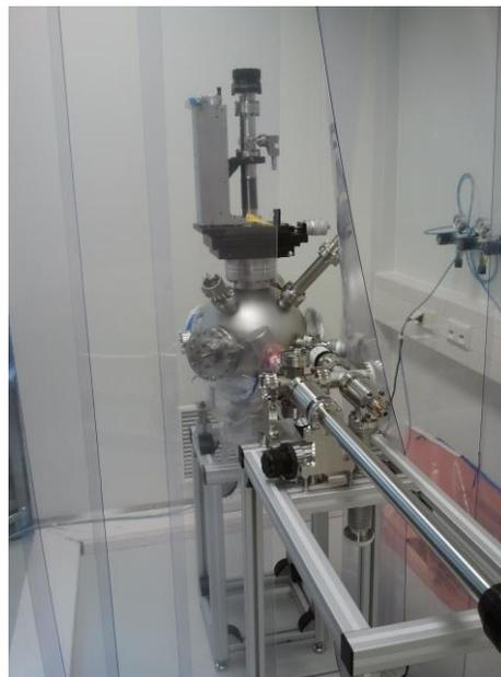
Figure 2: The GaAs preparation chamber in clean room. The magnet manipulator is used to install a new substratum.
