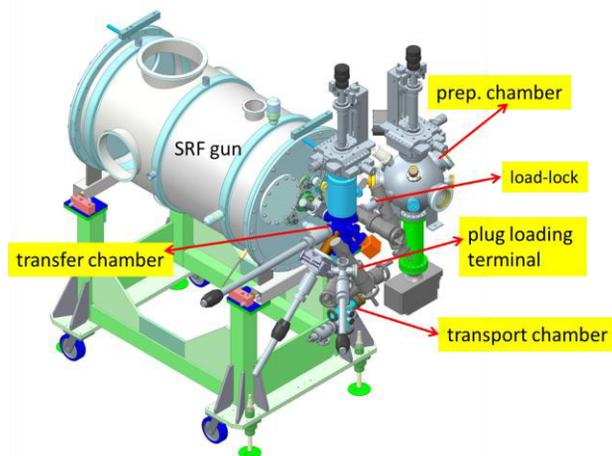
Figure 6: SRF gun with the new photocathode transfer system. The GaAs(Cs,O) will be in situ activated and then quickly transported into SRF gun.
