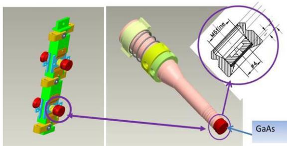
Figure 3: The design of new photocathode plug. Up to four plugs can be transported with this carrier. The plugs are fixed on the flags (in blue) with CuBe springs (in yellow) and the flags can be handled by magnet manipulator [8].
