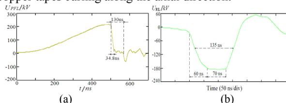
Figure 4: (a) The charge voltage waveform of the HBPFL; (b) The typical voltage waveform on the  $160 \Omega$  load.
