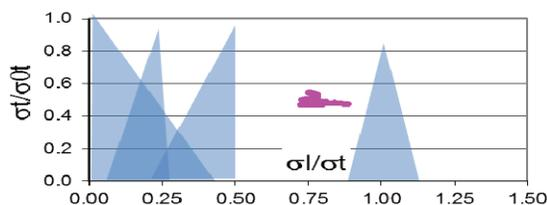
Figure 8: Hofmann coherent resonance diagram for the DTL.
