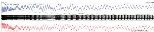
Figure 10: End-to-end simulation of the linac to 300 MeV at 50 mA.
