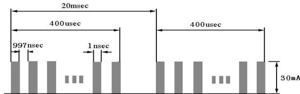
Figure 3: Time structure of micro-pulsed mode.
