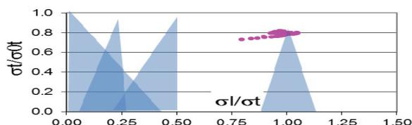
Figure 9 Hofmann coherent resonance diagram for the CCL.
