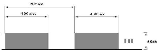
Figure 2: Time structure of the long-pulsed mode.
