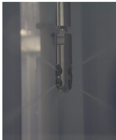
Figure 2: Spray head (6 nozzle design).
