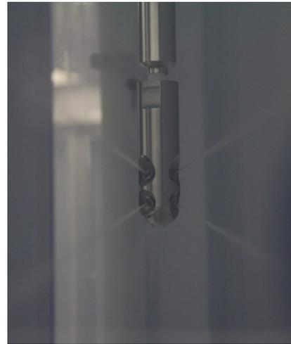
Figure 2: Spray head (6 nozzle design).
