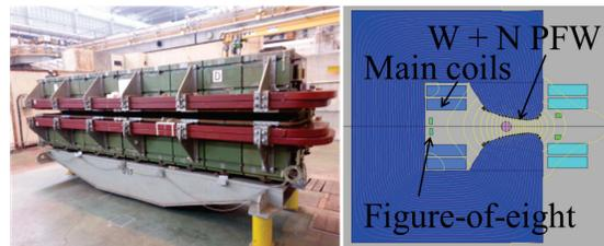
Figure 1: Left: Picture of one PS magnet. Right: Cross-section of PS magnet (“closed” type).
