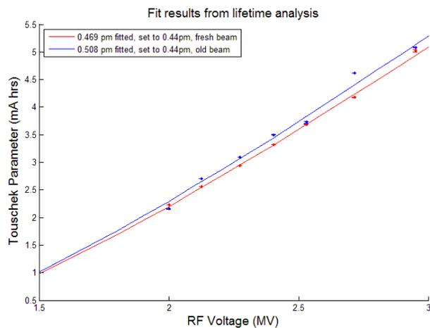
Figure 4: Lifetime analysis showing the effect of beam polarization. The blue data points were obtained using the exact same conditions as the red, except for waiting at least 15 minutes after injection. They show a longer lifetime, as expected and more noise in their distribution compared to the red data points of largely unpolarized beam.
