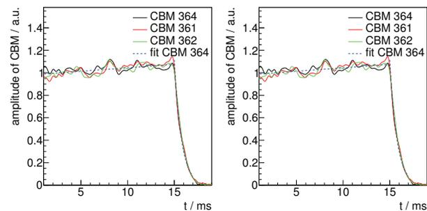
Figure 1: Grow/damp measurements at BESSY II. Left: Measurement in the horizontal plane during operation with near zero chromaticity. Right: Measurement in the longitudinal plane at nominal beam conditions.
