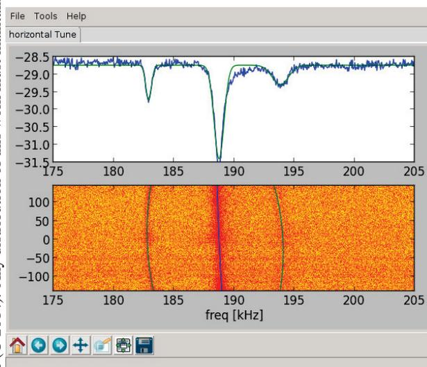
Figure 2: Control panel of bunch-by-bunch tune measurement in the horizontal plane. Top part shows averaged spectrum over all bunches, bottom part shows dependence over the multi-bunch part of the fill pattern. The side bands reveal a variation of synchrotron frequency over the bunch train due to transient beam loading.
