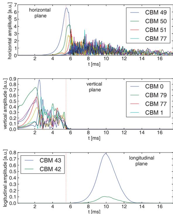
Figure 5: Captured partial beam-loss event at the MLS showing CBIs in all three dimensions. The beam-loss time is indicated by a vertical dotted line.
