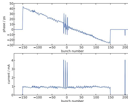
Figure 3: Top: Synchrotron phase gradient due to transient beam loading measured by the feedback system. Bottom: Typical hybrid-fill pattern.
