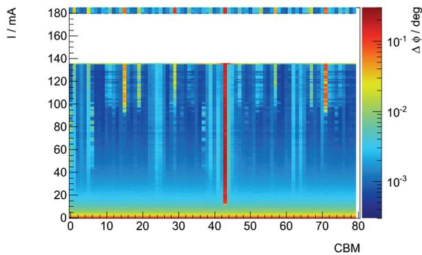
Figure 4: Measurement at the MLS showing the amplitude of the longitudinal coupled bunch modes vs. the total current stored in the ring. The dominating CBM 43 can clearly be seen. The horizontal gap is caused by a partial beam-loss during the scraper operation.
