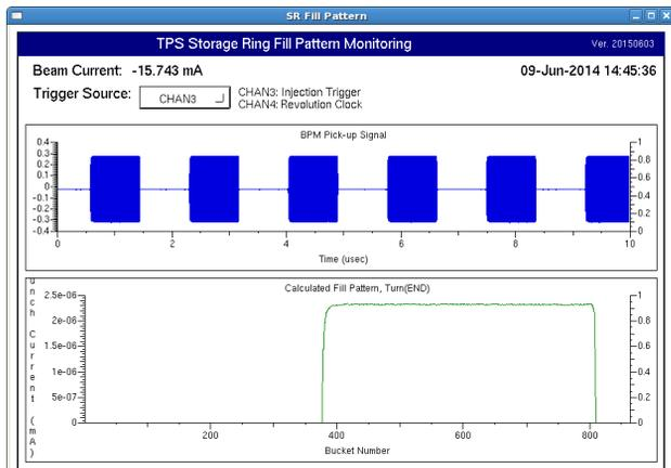
Figure 4: EDM page for the TPS storage ring fill pattern monitoring with the simulated signal.
