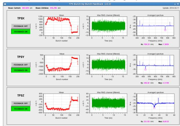
Figure 6: Operator interface to operate the bunch-by-bunch feedback system include transverse as well as longitudinal feedback system. Various waveforms include beam oscillation amplitude in RMS and bunch phase oscillation in RMS, are shown on the integrated with front-end and iGp control page.
