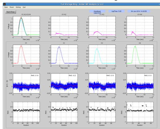
Figure 3: Kicker waveform analysis interface which was verified in the TLS.
