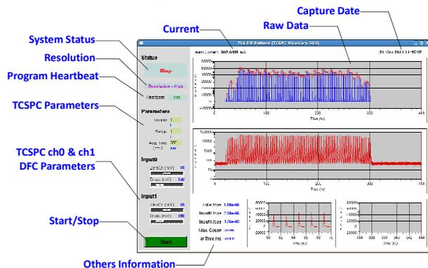
Figure 5: Layout of the TCSPC EDM page.
