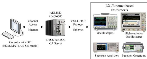
Figure 1: System architecture of building EPICS waveform support environment with LXI/Ethernet-based instruments.
