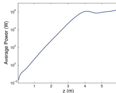
Figure 3: Average FEL power versus the distance (z) in the undulator.
