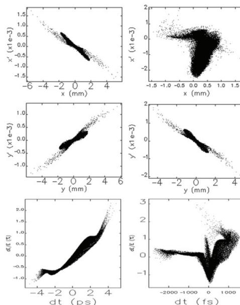
Figure 2: Horizontal (top), vertical (middle) and longitudinal (bottom) phase spaces before (left) and after (right) the magnetic chicane.
