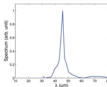
Figure 4: Spectrum of the FEL radiation at the distance 6 m in the undulator.
