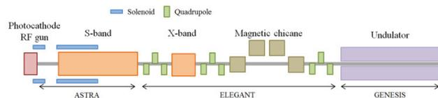
Figure 1: THz FEL linac for the ASL.
