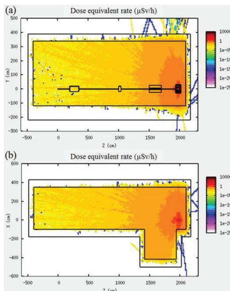
Figure 6: Dose equivalent during the beam time from FLUKA simulation in (a) side view and (b) top view.
