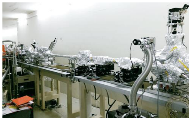
Figure 5: ID front end FE05 leak check and pumping in the tunnel.
