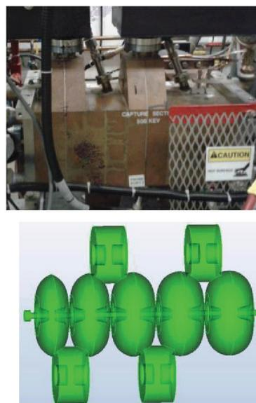
Figure 1: The old capture cavity and its simulation model.
