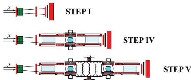
Figure 1: The MICE programme of staged construction and running. Step I (completed in 2013) consists of the muon beamline and particle identification. Step IV (first running expected in 2015) adds the spectrometers solenoids, trackers and first absorber focus coil module. Step V (first running expected in 2018) adds an RF coupling coil module and second absorber focus coil module.
