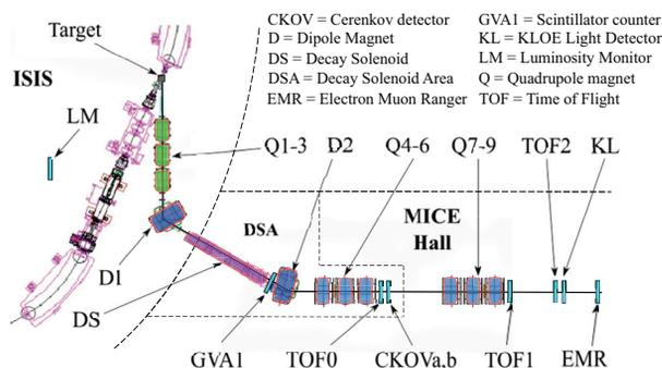
Figure 2: The MICE Muon Beamline, showing the beamline magnets and PID detectors. The far left shows part of the ISIS accelerator which serves as a proton driver, with a titanium target used to generate pions by intercepting the circulating proton beam.
