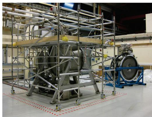
Figure 4: The two AFC modules at RAL. Different absorber materials may be used interchangeably.
