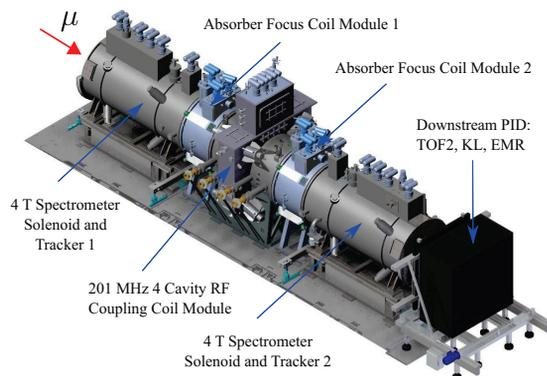
Figure 3: The MICE Step V Cooling Channel sandwiched by the up- and downstream spectrometers.
