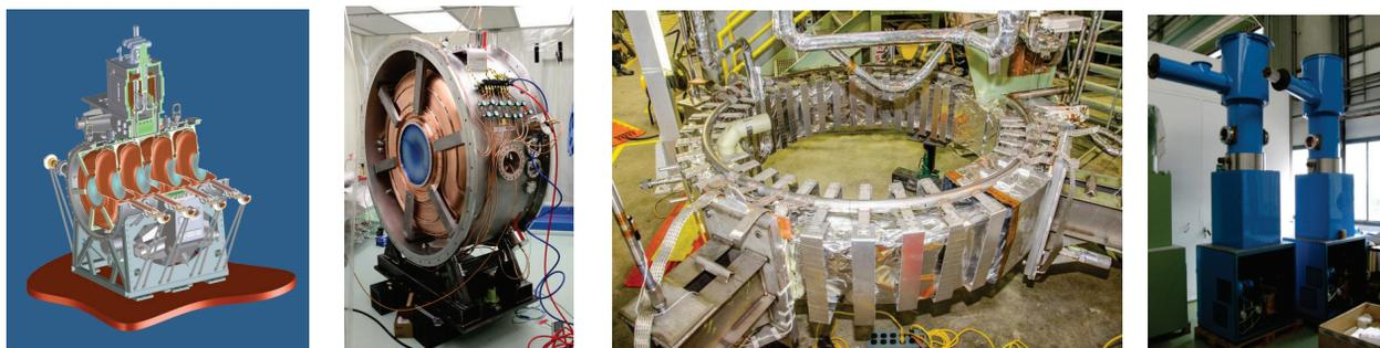
Figure 5: *Left*: Cutaway CAD drawing of the four cavity RFCC module. *Centre-left*: A MICE 201 MHz RF cavity. *Centre-right*: CC cold mass under test at Fermilab. *Right*: Two 201 MHz RF power supplies undergoing refurbishment at Daresbury Laboratory.
