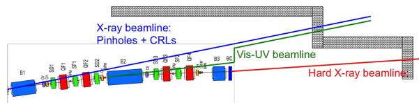
Figure 1: Schematic drawing of the possible beamlines in Sirius coming from 3 dipoles, B1, B2 and BC respectively.
