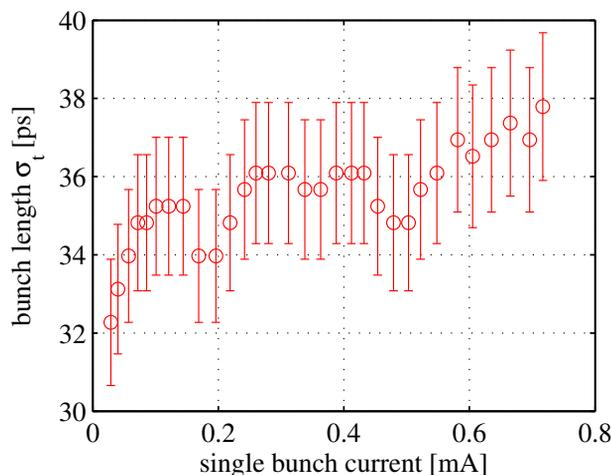
Figure 5: Measurement of the natural bunch length with reflective input optics and constant light intensity in the streak camera (cavity voltage 1.8 MV).
