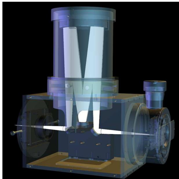
Figure 1: Offner relay system for streak camera reflective input optics. SR is beam focussed on the entrance slits on the right and focussed onto the cathode on the left.
