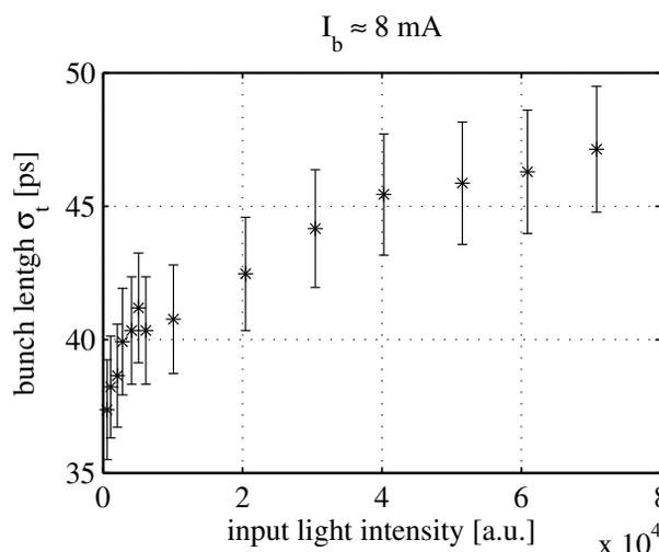
Figure 2: Variation in the measured bunch length against the input light intensity into the streak camera. Bunch current was kept constant and the intensity modified with an ND filter.
