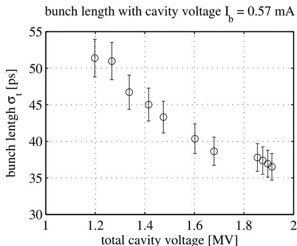
Figure 6: Bunch length against cavity voltage.
