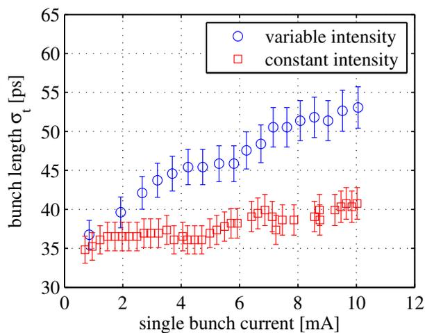
Figure 3: Comparison between fixed and variable light intensity on the streak camera.
