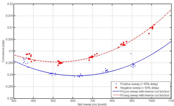
Figure 4: Non-linear calibration curve for the streak camera. Note the difference in the calibration curves between the different sweep directions. The cause might be a result of distortions on the RF input that drives the synchroscan.
