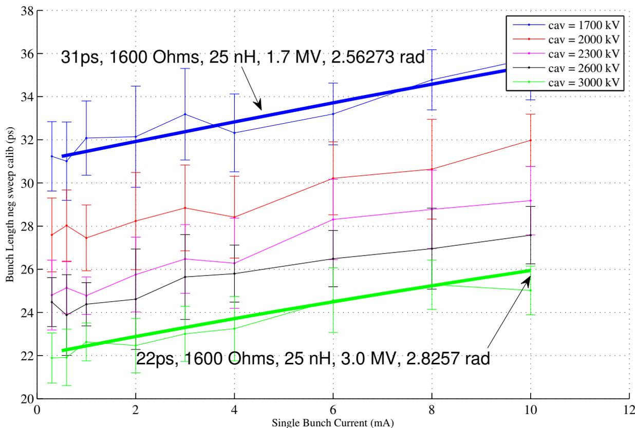
Figure 7: Estimation of the storage ring impedance.
