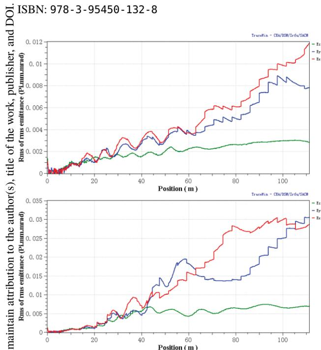
Figure 3: The nominal emittance evolution (the upper picture) and the corrected one (the lower picture) with error analysis after the solenoid failure in the middle part of the Spoke021 section.
