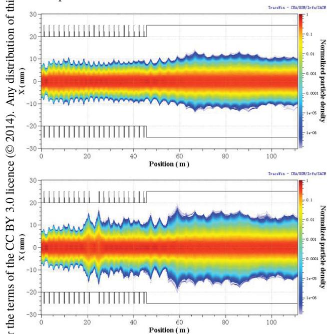
Figure 4: The nominal particle trajectory (the upper picture) and the corrected one (the lower picture) with error analysis after the solenoid failure in the middle part of the Spoke021 section.
