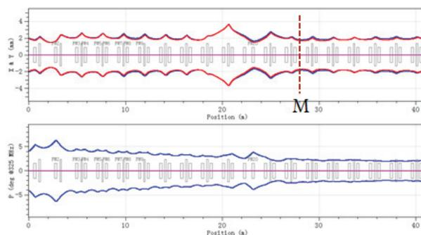
Figure 2: Envelope in the Spoke021 section in both transverse and longitudinal plates and the longitudinal phase section also been shown after the rematch of the solenoid failure in the low energy section.
