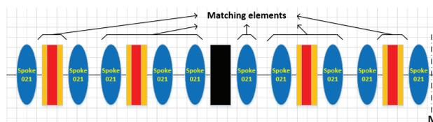
Figure 1: Rematch method for a solenoid failure in the middle part of the Spoke021 section.
