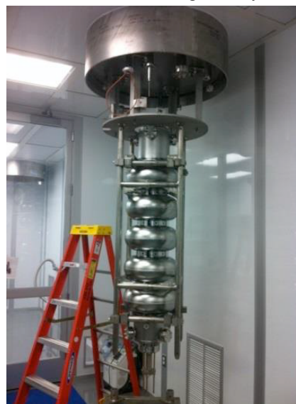
Figure 5: 704 MHz cavity manufactured by AES at vertical test facility.
