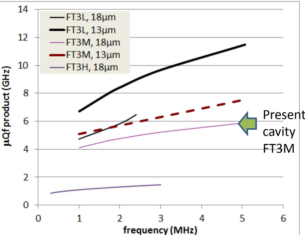
$$\mu Q f \propto \text{shunt impedance}$$
