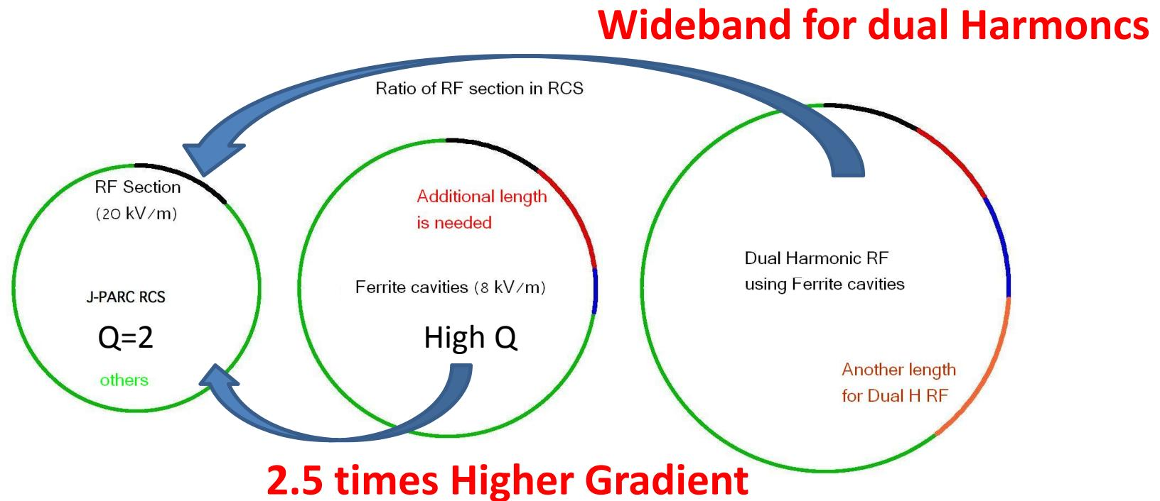
For MR upgrade, higher gradient cavity for high rep. rate ( $\sim 1\text{Hz}$ ) is necessary as space is limited.
