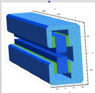
Permanent magnet ( $\text{Sm}_2\text{Co}_{17}$ ) dipoles
