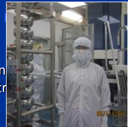
Dr. Zhai Ji Yuan and Cavity IHEP-01 before high pressure water rinsing in class-100 clean room at IHEP
