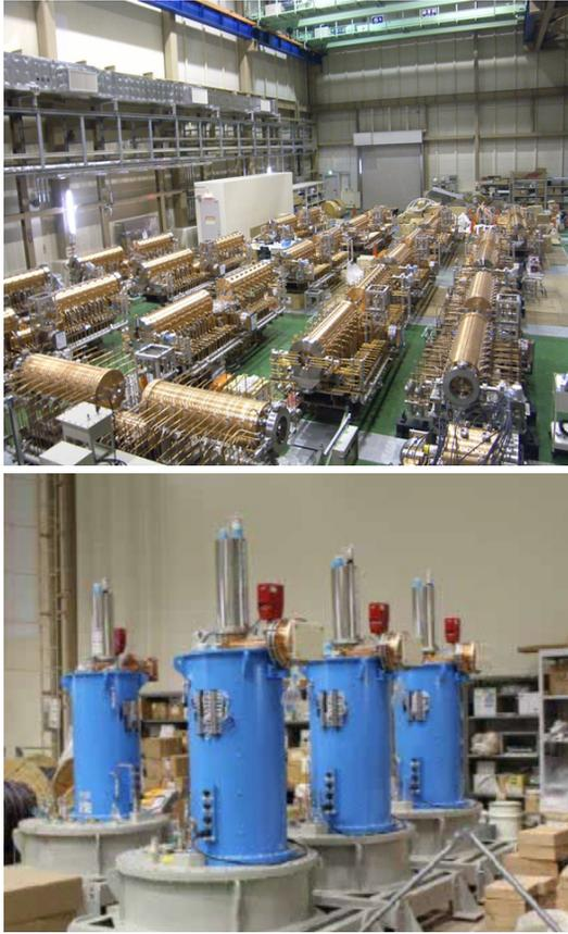
Figure 10: ACS cavities (upper) and 972MHz klystrons (lower) waiting for the installation.
