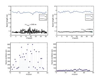
Figure 6: Bunch length (top) and bunch position oscillations (bottom), at flat top, for the bunches of a single batch 50 ns LHC beam, for Q26 (left) and for Q20 (right) [27].
