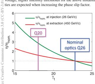
Figure 4: Slippage factor  $\eta$  relative to the value of the nominal optics (nominal  $\gamma_t = 22.8$ ) as a function of  $\gamma_t$  [26].
