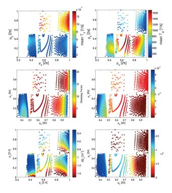
Figure 3: Analytical parameterization of the TME cell phase advances with the IBS horizontal (top, left) and longitudinal (top, right) growth rates, the detuning factor (middle, left), the momentum compaction factor (middle, right), the horizontal chromaticity (bottom, left) and the Laslett tune shift (bottom, right) [19].
