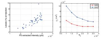
Figure 5: Losses at SPS injection as a function of the extracted PS intensity [28] (left) and ECI thresholds for various intensities comparing the nominal (red) with the low  $\gamma_t$  SPS optics (blue) [31] (right).
