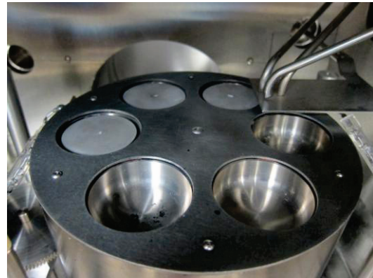
Figure 1: Niobium samples on the sample holder in the PLD chamber.
