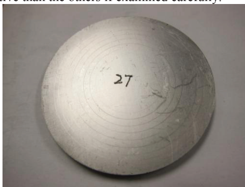
Figure 2: A niobium sample with laser polished rings on the surface.
