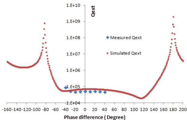
Figure 7: Comparison of measured external  $Q$  factor and simulation results.
