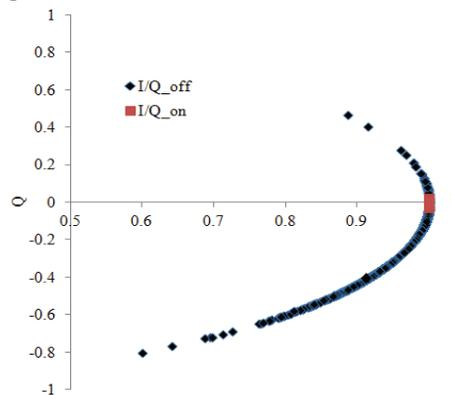
Figure 5: Field stability with I/Q loop.
