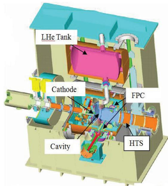
Figure 1: ERL SRF gun cryomodule.
