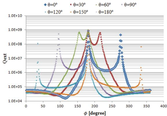
Figure 6: The external  $Q$  factor change with one phase shifter at different initial states.
