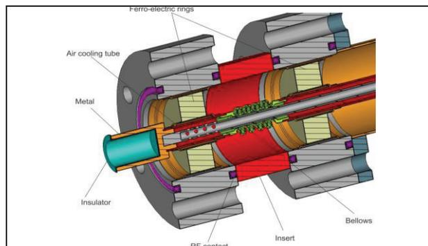
Figure 4: 3D CAD model of the phase shifter.
