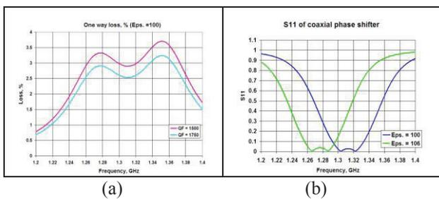
Figure 3: Simulations of loss factor vs. frequency for the coaxial tuner containing two low permittivity ferroelectric rings; (a) phase shift vs. frequency; (b) S11 parameters of the coaxial phase shifter  $\epsilon = 100$ .
