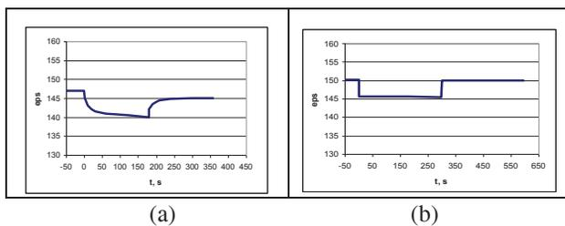
Figure 6: Dielectric response measurement (dielectric constant) after the rectangular dc bias pulse: (a) before annealing  $\epsilon \sim 150$ ; (b) after annealing.
