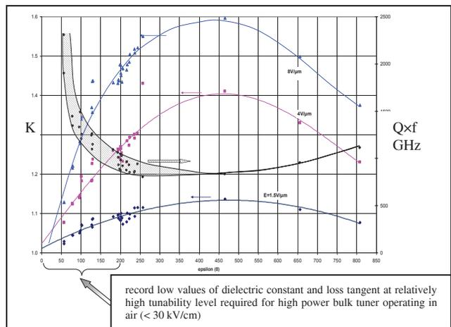
Figure 1: BST(M) ferroelectric tunability dependence on the DC field magnitude.
