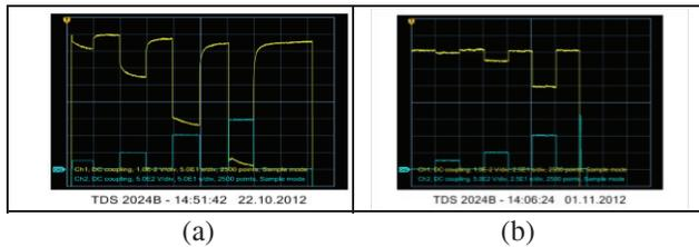
Figure 5: Measurement results of the switching time of ferroelectric ceramic samples with Au electrodes deposited; response of the ceramic samples (yellow) to a pulsed electric field (blue): (a) before and (b) after the annealing.
