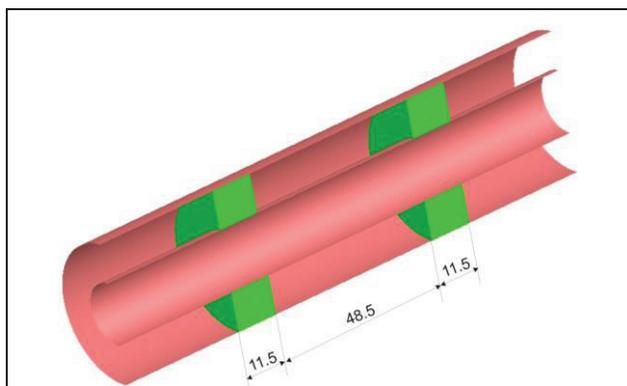
Figure 2: Geometry (units in mm) of the coaxial phase shifter containing two ferroelectric rings with low zero-field dielectric constant  $\epsilon = 100$ .
