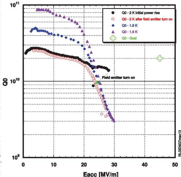
Figure 5: First test result of 1-cell 1300 MHz large-grain niobium cavity G2 processed with mirror-finish mechanical polishing, heat treatment and electropolishing.
