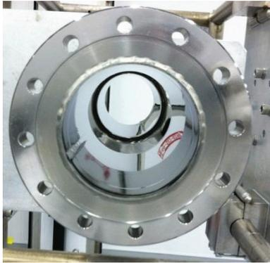
Figure 4: The view of a 1-cell 1300 MHz large grain niobium cavity mechanically polished to mirror finish. The red arc area at 4-5 o'clock is the reflection of a red tape on the clean room wall pointing a fire extinguisher.
