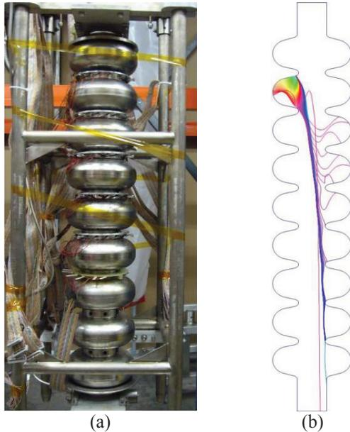
Figure 1: (a) A nine cell ILC cavity equipped with cryogenic radiation detection diodes for field emitter localization; (b) Trajectories of electrons emitted from the location as determined by the JLab procedure.
