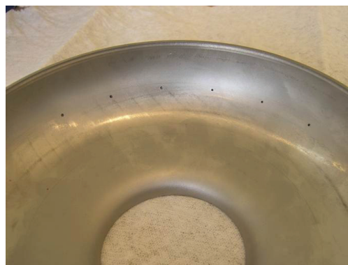
Figure 1: Half cup of the pit cavity after drilling of the pits.
