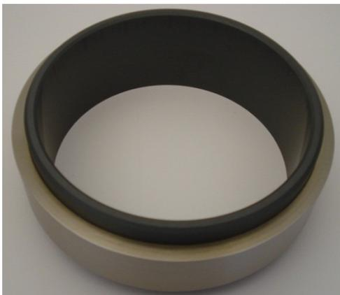
Figure 5: Silicon carbide ring shrink-fitted into a titanium grade 5 cylinder. After 2 thermo-cycles to 77 K neither visible damage nor loosening was observed.
