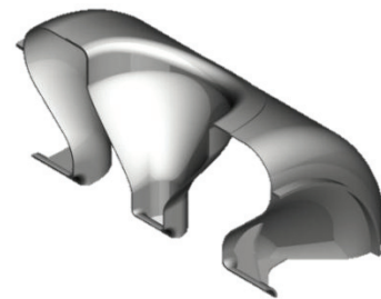
Figure 7: One quarter CAD model of the SSR2 resonator.
