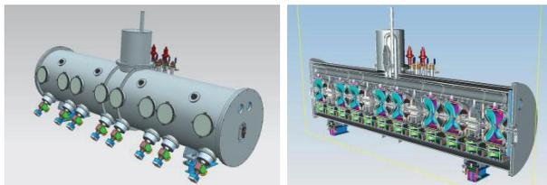
Figure 4: A view of the SSR1 cryomodule.
