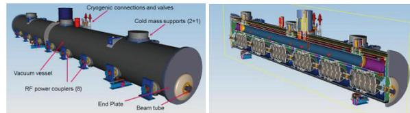
Figure 5: 650 MHz cryomodule conceptual design.
