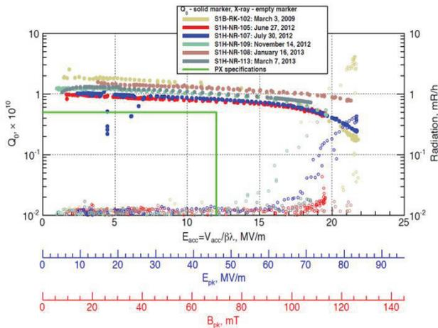
Figure 3: SSR1 bare cavity test performance.
