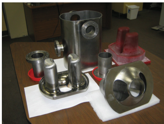
Figure 4: All cavity parts before welding.
