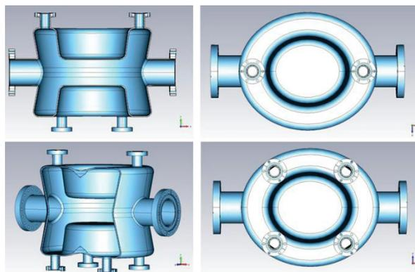
Figure 1: Geometry of the double quarter wave cavity.
