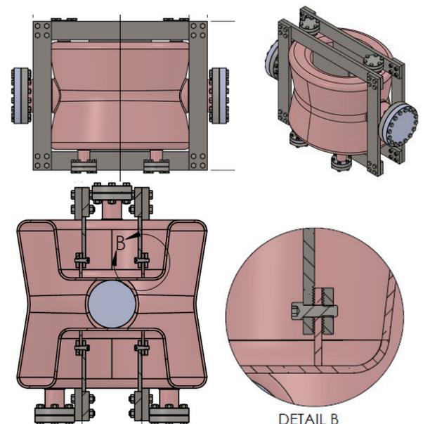
Figure 6: Geometry of the double quarter wave cavity with stiffeners.
