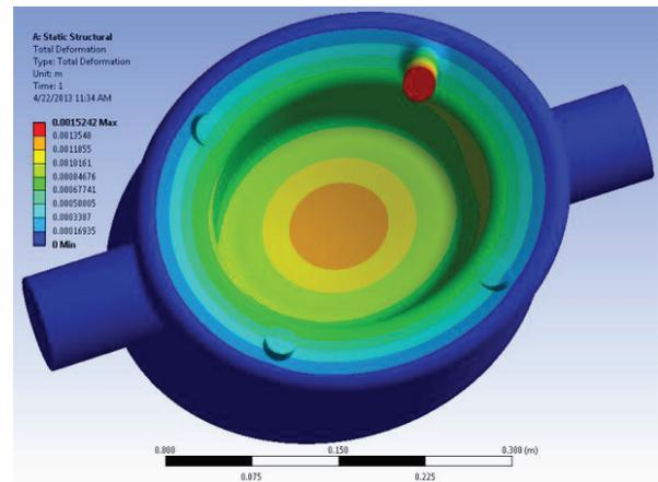
Figure 4: Cavity deformation without stiffeners.
