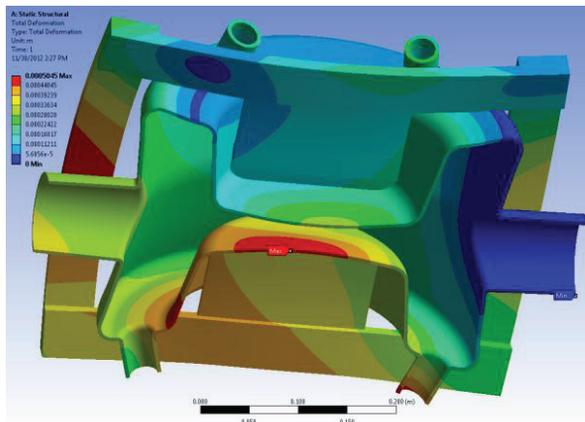
Figure 7: Cavity deformation with stiffeners.
