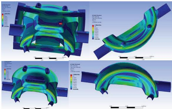
Figure 8: Cavity stress with stiffeners.
