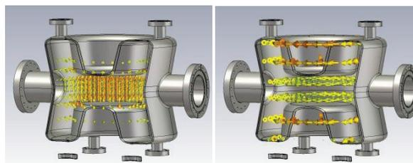
Figure 2: Electric field (left) and magnetic field (right) of the fundamental mode.
