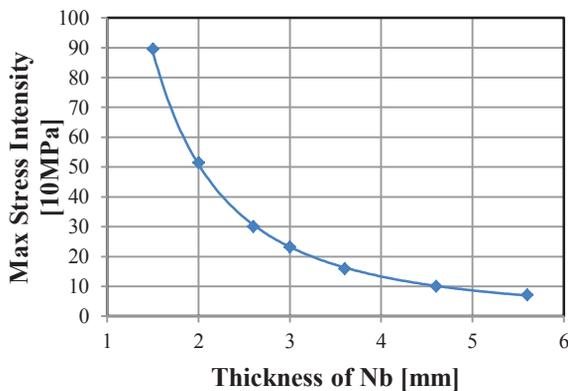
Figure 3: Crab cavity maximum stress intensity vs Nb thickness.
