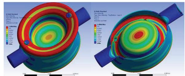
Figure 5: Cavity stress without stiffeners. Red color indicates area with stress higher than the maximum allowable stress at 70 MPa.
