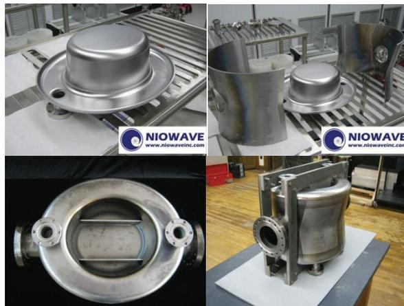
Figure 9: Fabrication of the double quarter wave crab cavity.
