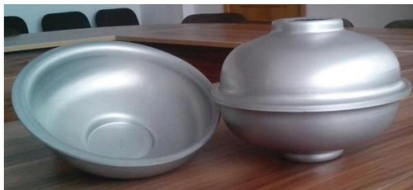
Figure 5: First half-cells made of aluminium by hydraulic deep drawing in Minsk.
