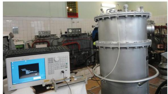
Figure 3: Stand for RF-tests at 4.2 K.
