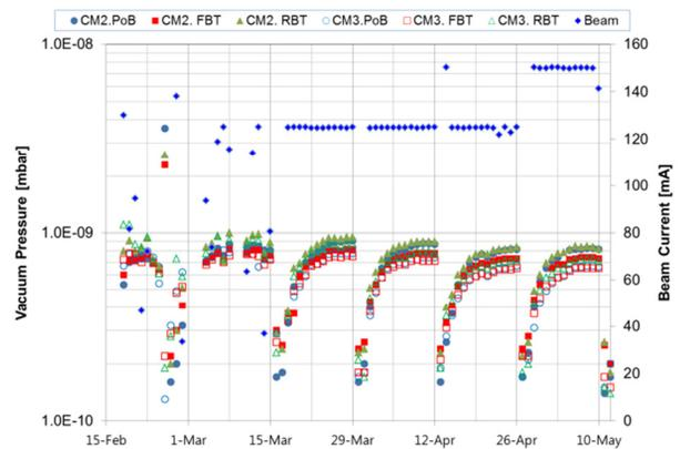
Figure 7: Vacuum pressure of windows (PoB) & cavities (RBT, FBT) and beam current.
