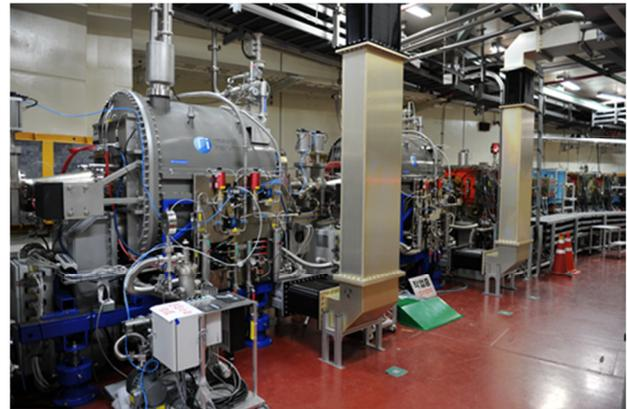
Figure 1: Two SRF modules in tunnel.
