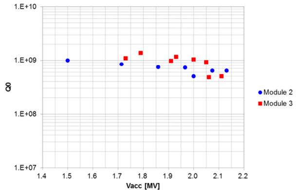
Figure 3: Measured Q0 with accelerating voltage.
