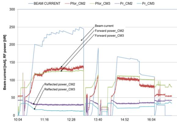
Figure 5: Short history of beam commissioning with two SRF cavities.
