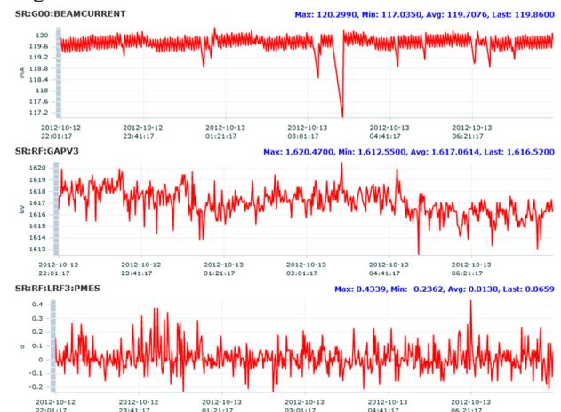
Figure 4: RF stability with 1<sup>st</sup> SRF cavity: middle-amplitude ( $\Delta V/V \sim 0.4\%$ ), lower-phase ( $\Delta \Phi/\Phi \sim 0.5^\circ$ ).
