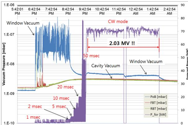
Figure 2: Vacuum pressure and forward RF power during commissioning 1<sup>st</sup> SRF module by RF power only.
