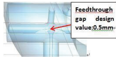
Figure 8: Definition of feedthrough gap.
