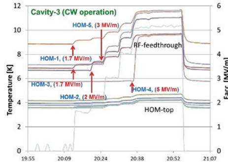
Figure 9: Observation of temperature rises at RF feedthroughs of HOM couplers due to quench at the Nb antenna tip.
