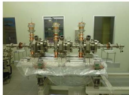
Figure 1: String assembly of three 2-cell cavities with six input couplers in a class-10 clean room.
