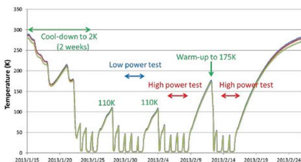
Figure 3: Cavity temperature during cool-down tests.
