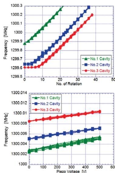
Figure 4: Tuner performance by a slide-jack tuner (top) and a piezo tuner (bottom).
