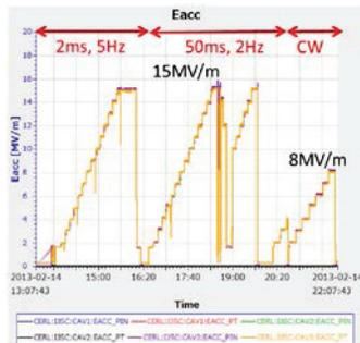
Figure 5: Accelerating gradient ( $E_{acc}$ ) during high power RF conditioning in Cavity-3 at 2 K.
