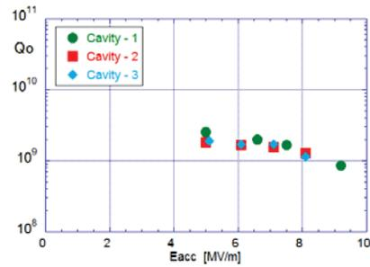
Figure 8: Measured  $Q_o$  values of three cavities in a CW operation at 2 K.
