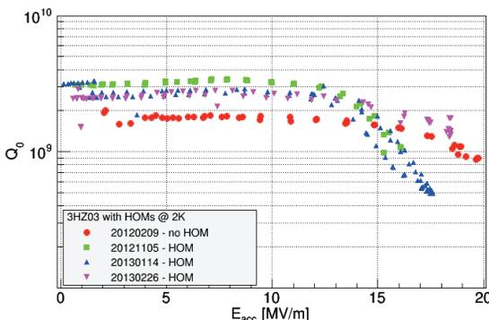
Figure 4: 3HZ03  $Q_0$  vs.  $E_{acc}$  with HOM pickups installed. For comparison, we have included the measurement without HOM of figure 3. The first two tests with HOM showed a strong field emission starting from 13 MV/m.
