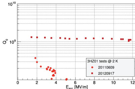
Figure 1: Cavity 3HZ01 test at LASA  $Q_0$  vs.  $E_{acc}$  in first test (red dots) and after retreatment (red squares).
