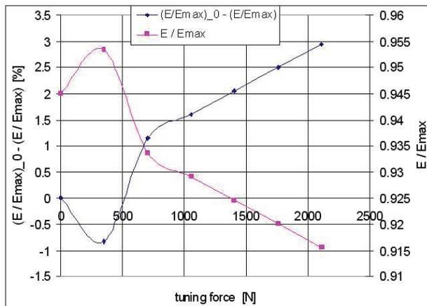
Figure 8: Electrical field profile change by gun cavity tuning.
