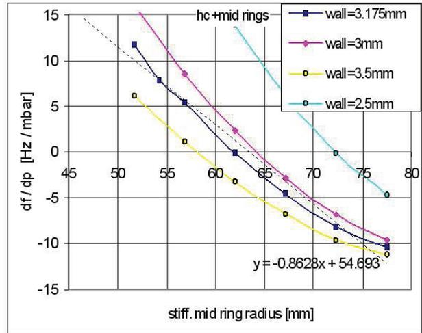
Figure 5: Simulation results of gun cavity and choke structure frequency shift under 1 bar external pressure depending on resonator mid-ring position.
