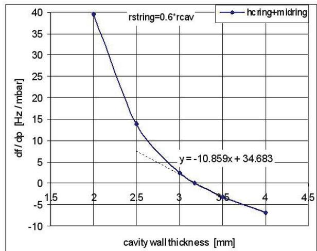
Figure 6: Simulation results of gun cavity and choke structure frequency shift under 1 bar external pressure depending on resonator wall thickness.
