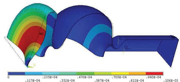
Figure 2: Cavity deformations under 1 bar external pressure.
