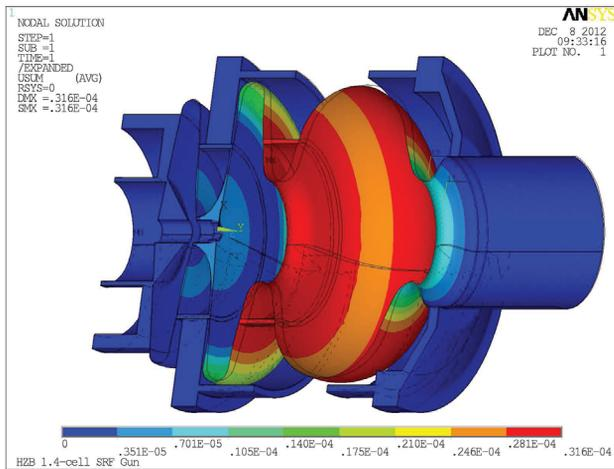
Figure 4: Deformations of gun cavity and choke structure in helium vessel under 1 bar external pressure.
