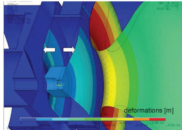
Figure 9: Deformations of gun cavity and choke structure without mid-cell ring in helium vessel under 1 bar external pressure.
