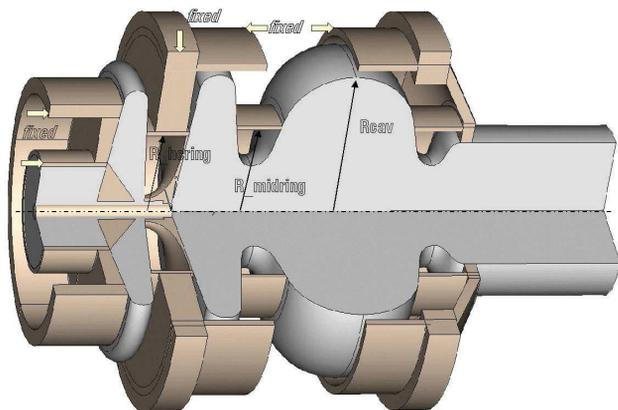
Figure 3: SRF gun simulation model.
