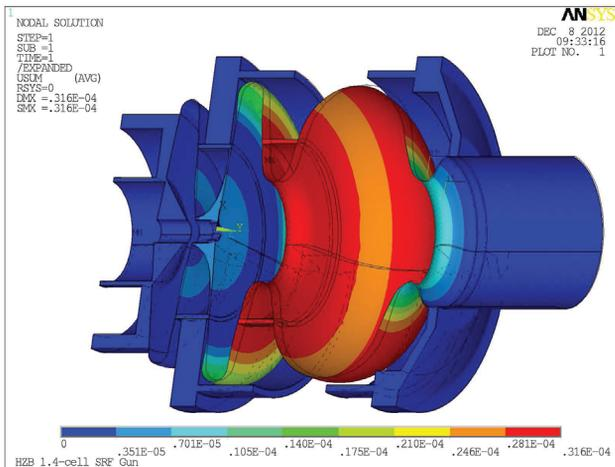
Figure 4: Deformations of gun cavity and choke structure in helium vessel under 1 bar external pressure.
