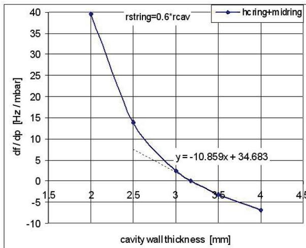
Figure 6: Simulation results of gun cavity and choke structure frequency shift under 1 bar external pressure depending on resonator wall thickness.
