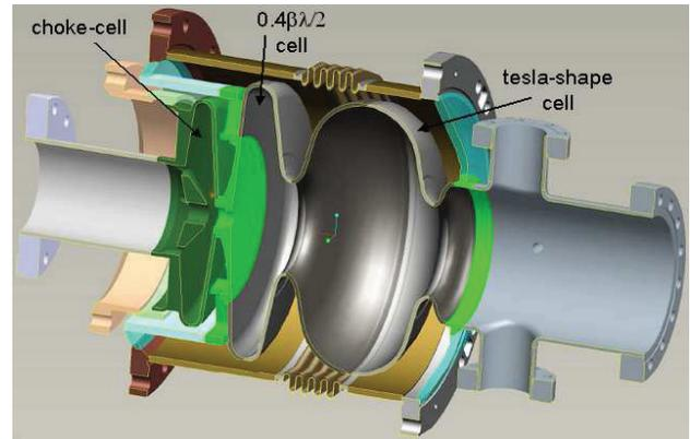
Figure 1: Schematic view of HZB BERLinPRO SRF gun cavity in helium vessel.
