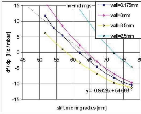
Figure 5: Simulation results of gun cavity and choke structure frequency shift under 1 bar external pressure depending on resonator mid-ring position.
