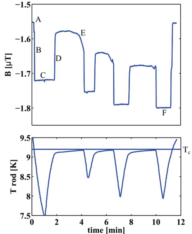
Figure 4: Behavior of trapped flux (FM1) and temperature upon heating in  $B_{\text{HC}} = 33 \mu\text{T}$ .
