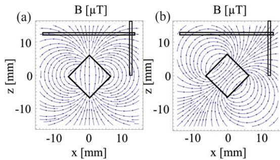
Figure 3: Magnetic field distribution for a constant magnetization of the niobium rod in  $z$ -direction (a) and tilted by  $45^\circ$  (b). The black rectangle indicates the positions of FM1 and FM3.
