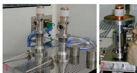
Figure 2: Warm (1) and cold (2) parts after ceramic integration and EB welding of inner and antenna.
