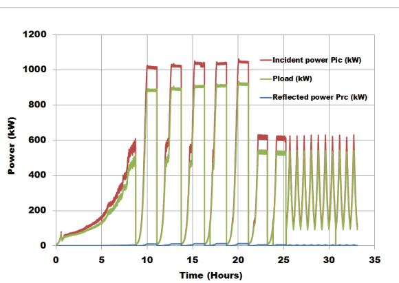
Figure 6: XFEL power coupler RF conditioning.
