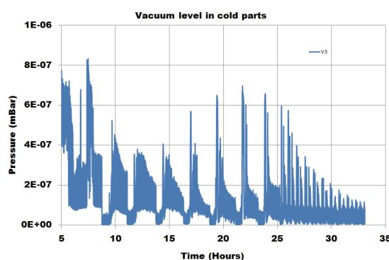
Figure 7: Pressure level measurements in cold parts during RF conditioning.
