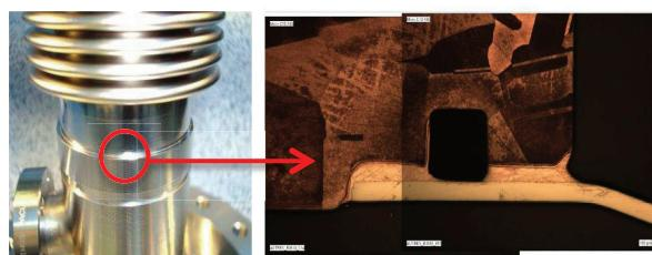
Figure 1: Cross section of a bellow-tube brazing junction.
