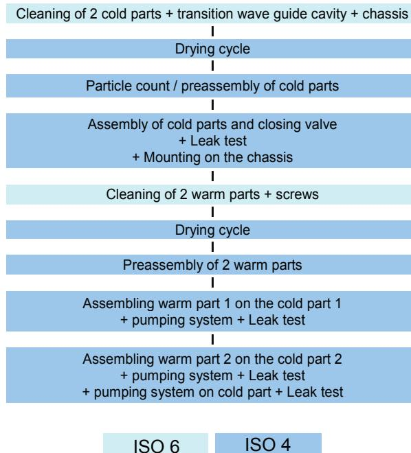
Figure 3: Coupler cleaning & assembling procedures in clean rooms.
