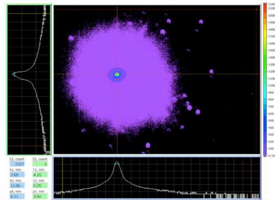
Figure 3: Top: measured beam transverse profile by using the OTR beam viewer. The beam size is  $\sim 50\mu\text{m}$  (rms) based on best Gaussian fit to the horizontal and vertical projections. Bottom: a high dynamic range beam profile measured with Ce:YAG showing beam halo around the core (vertical scale is logarithmic).
