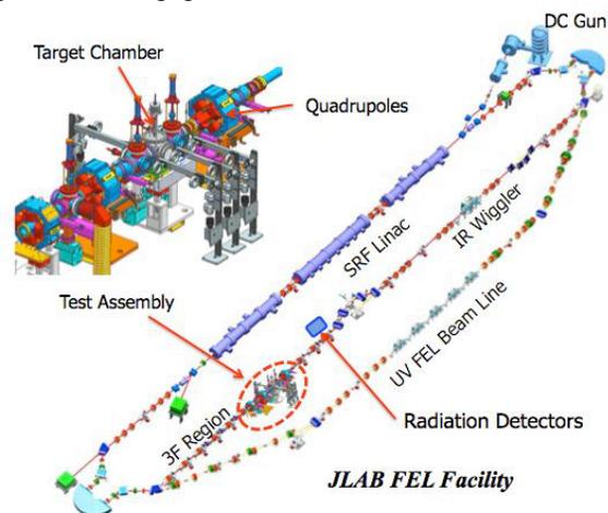
Figure 1: A schematic of the JLAB FEL Facility showing the ERL accelerator, IR and UV FEL beamlines, the proposed beam transmission test experiment assembly and its location. The location of the radiation detectors is also shown.
