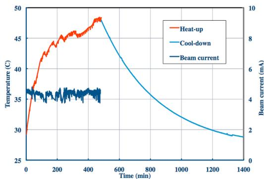
Figure 4: Beam block temperature and beam current vs. run time when transmitting a 4.5mA/100MeV beam through the 2 mm hole. After the beam is turned off, a cool-down curve is recorded and shown here.
