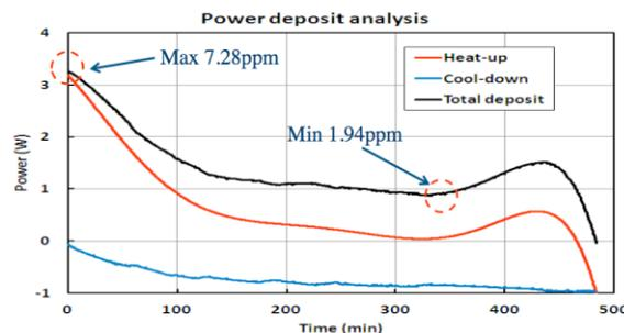
Figure 5: Analysis of beam power deposited into the beam block through 2 mm beam tube test based on data in Fig. 4.
