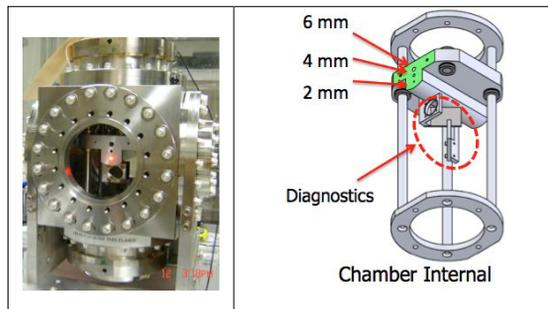
Figure 2: Left: A photo of the target chamber with three beam tubes and diagnostics seen from an open side port. An aligning laser beam spot can be seen on the 2 mm hole. Right: 3D illustration for the internal components and mechanical structure of the target.
