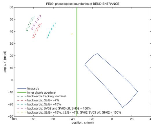
Figure 7: Dipole beamline: phase space boundaries at the entrance to the bending magnet in the worst combination of errors.
