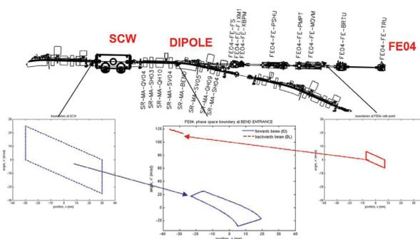
Figure 1: Section of the storage ring used for the tracking studies in the case of an ID beamline. Initial phase-space coordinates for the forwards tracked beam (bottom left), for the back tracked beam (bottom right) and final distributions (bottom centre) are shown: in this example the two distributions do not overlap, indicating a safe situation.
