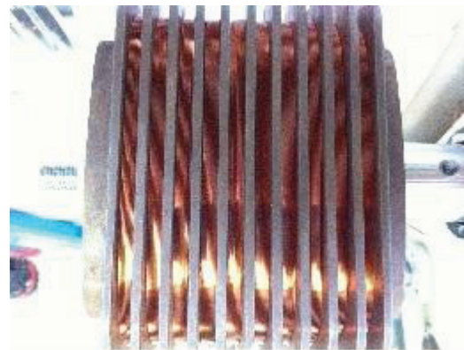
Figure 3: Photo of the five periods prototype SCU wound with copper wires.
