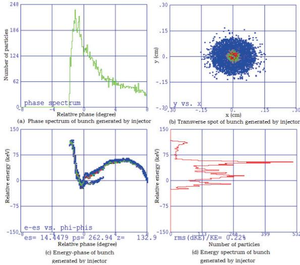
Figure 7: Energy spectrum, size, length of beam.
