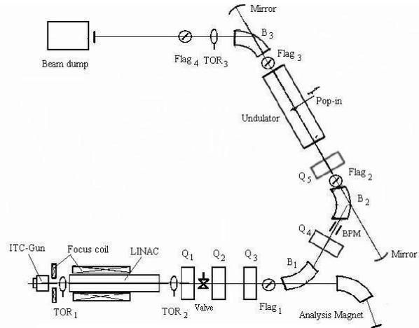
Figure 1: Layout of THz facility.
