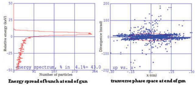
Figure 4: Energy spread and phase space at end of the gun.
