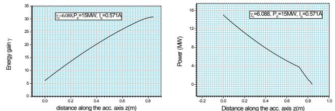
Figure 5: Energy gain curve and power distribution in LINAC.
