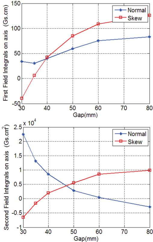
Figure 3: The integras of magnetic field with the magnet field gap (zero phase shift)
