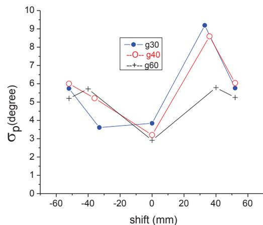
Figure 2: The radiation phase error with the magnet field phase shift for different magnet gap
