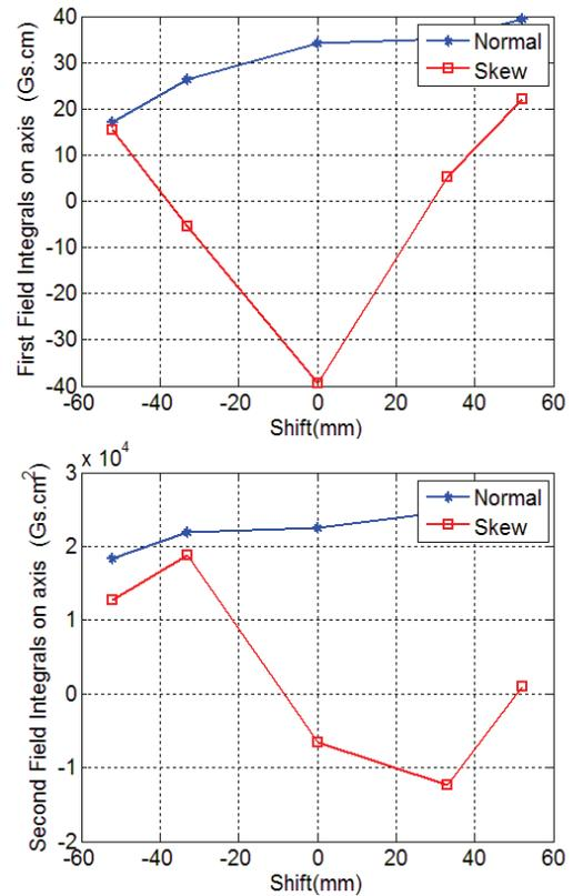
Figure 1: The field integrals with phase shift at the minimum magnetic gap
