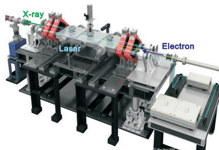
Figure 2: Drawing of the LCS collision point.
