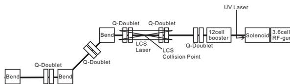
Figure 1: Schematic of LCS experimental setup at LUCX.
